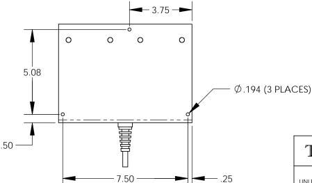
NOTE: BUMPER FEET REMOVED IN THIS VIEW TO SHOW MOUNTING HOLES.
