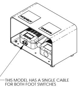
ENCLOSURE RATING: UL/CSA/NEMA ENCLOSURE TYPE 1 IEC 60529 IP 21
