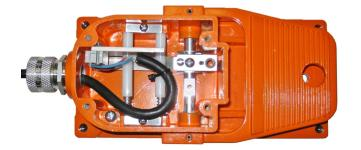
**Cable routing:** Route cable and solder wires to potentiometer in U shape, as shown (so as to assist in soldering leads to terminals). Secure with cable tie so wires cannot contact moving parts. Picture shows model G700-1K (note: this picture does not show the switch that is on the "-S" versions).
